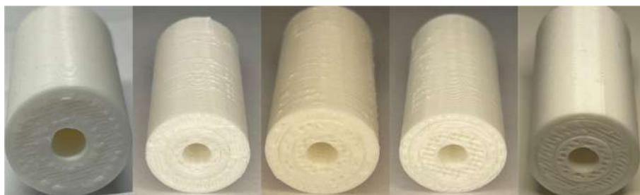
Figure 1. Fuel grains with different infill density gradients. From left to right: T100, T252252, T333333, T512424, T334520.
